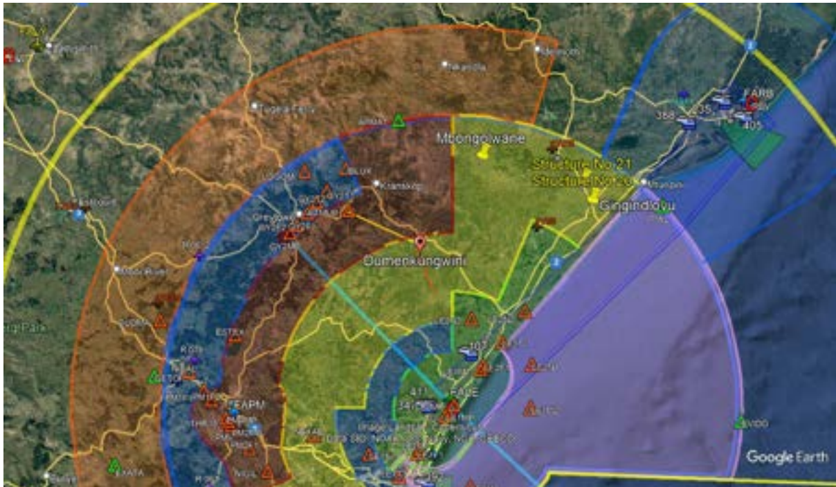
Figure 1. 31: Showing the Gingindlovu-Mbongolwane 132kV powerline deviation site with relation to nearest airport at Eshowe Airport at 16km away and Isithebe Airport located 17 kilometres away according to ATNS.
