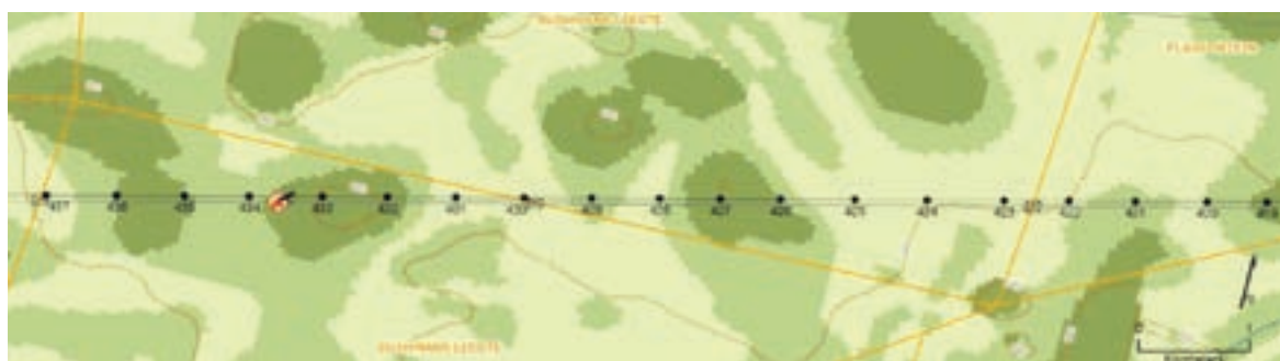
Figure 1: Example of an environmental sensitivity map in the context of a final overhead transmission and distribution profile
